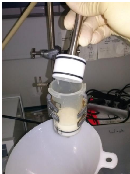
Figure 3: Filling the column with water
