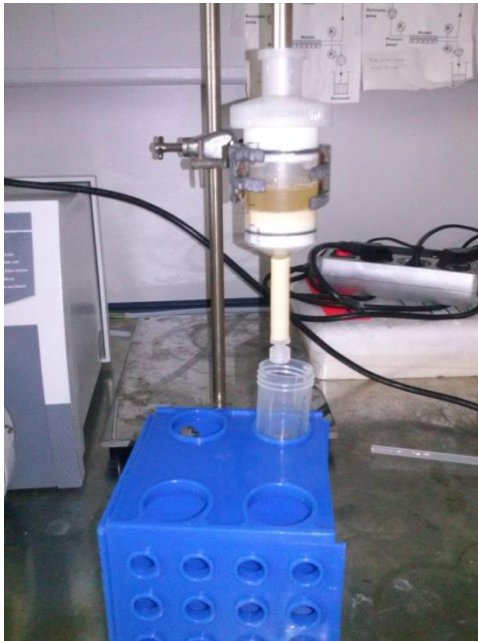
Figure 6: MAF column filled with elution buffer, outlet is closed with a plugged rubber tube
